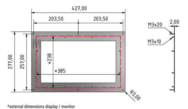
stainless steel frame with countersunk holes M4
