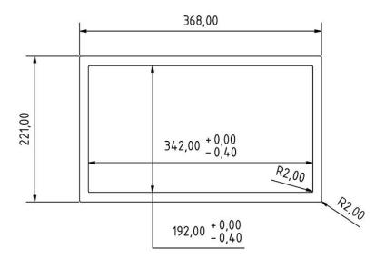
VSG safety glass 6 mm for 2 mm front panel Acrylic glass 4 mm for 2 mm front panel
