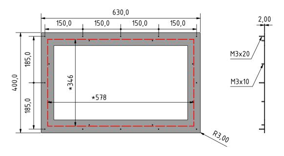
stainless steel frame with countersunk holes M4
