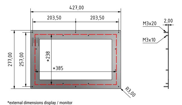
stainless steel frame with countersunk holes M4
