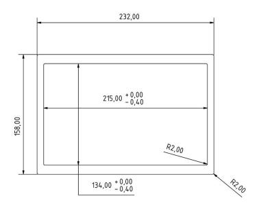
VSG safety glass 6 mm for 2 mm front panel Acrylic glass 4 mm for 2 mm front panel
