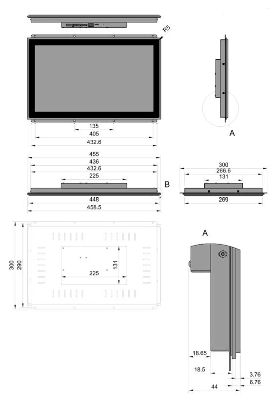
The touch sensor is designed and calibrated for use with a 6mm glass panel in front of the screen. If the display is installed behind an existing glass panel (e.g. glass tableau), the VSG glas panel shown on the drawings in this document is not needed.
